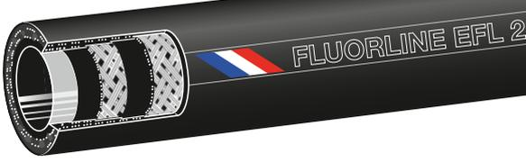
**FLUORLINE** universal pump hose for chemicals, petroleum based products, for propane, butane and other L.P. gases, as well as solvents as per resistance chart overleaf. Meets EN 1360 LT.
